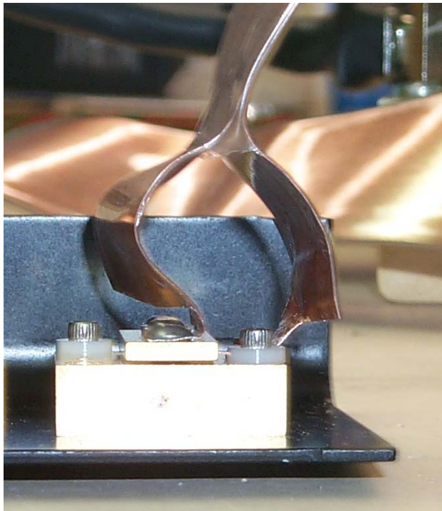
Figure 4 - Stripline Connection To Laser Diode
